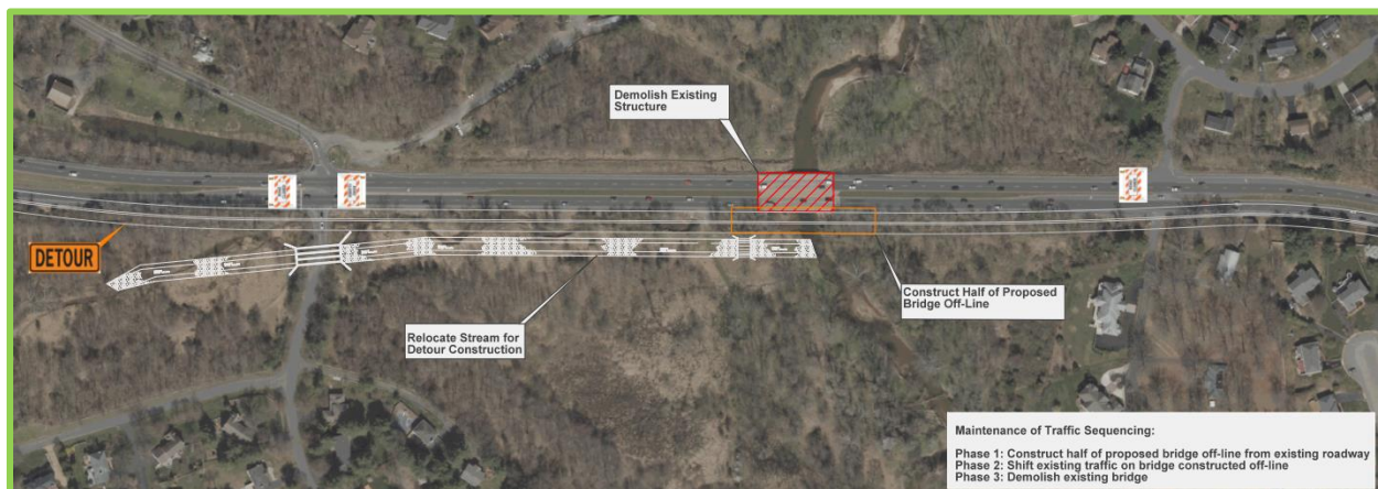
Figure 2-9: Route 7 Widening Option with New Bridges at Existing Bridge Location Maintenance of Traffic
