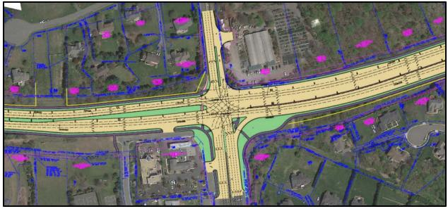
Figure 3: Revised Typical Section of the At-grade Intersection of Route 7 at Baron Cameron Ave / Springvale Road
