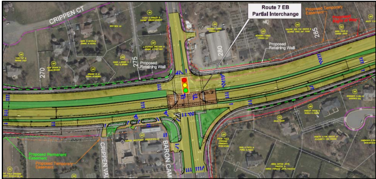
Figure 1: Public Hearing Conceptual of the Partial Interchange of Route 7 at Baron Cameron Avenue / Springvale Road
