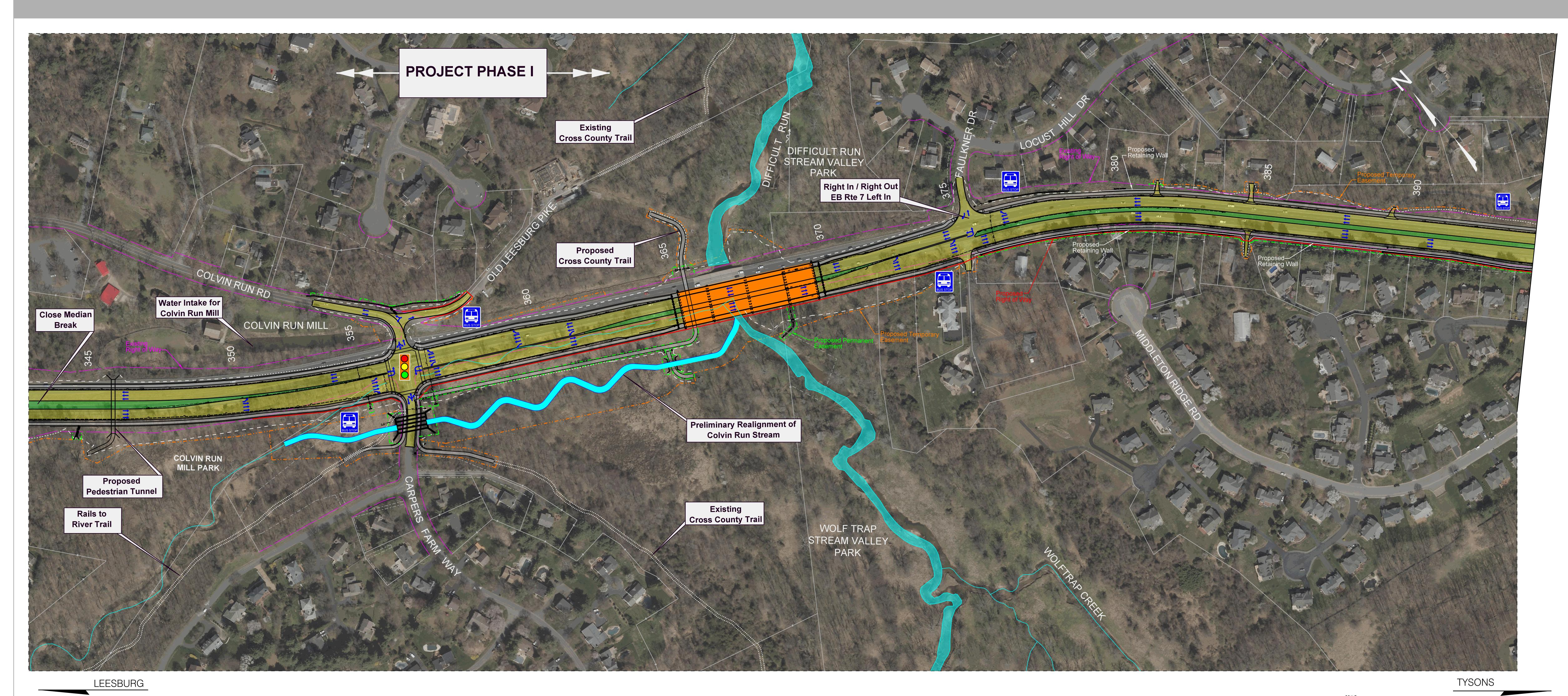
Legend Proposed Road ----- Construction Limits in Cut – – Construction Limits in Fill Proposed Bridge Proposed Shared Use Path/Sidewalk/Trail ··-··- Proposed Temporary Easement Proposed Preliminary Stormwater Management Basin ---- Proposed Permanent Easement Existing Bus Stop Location (Location to be revised with Proposed Design) **Existing Right of Way**
