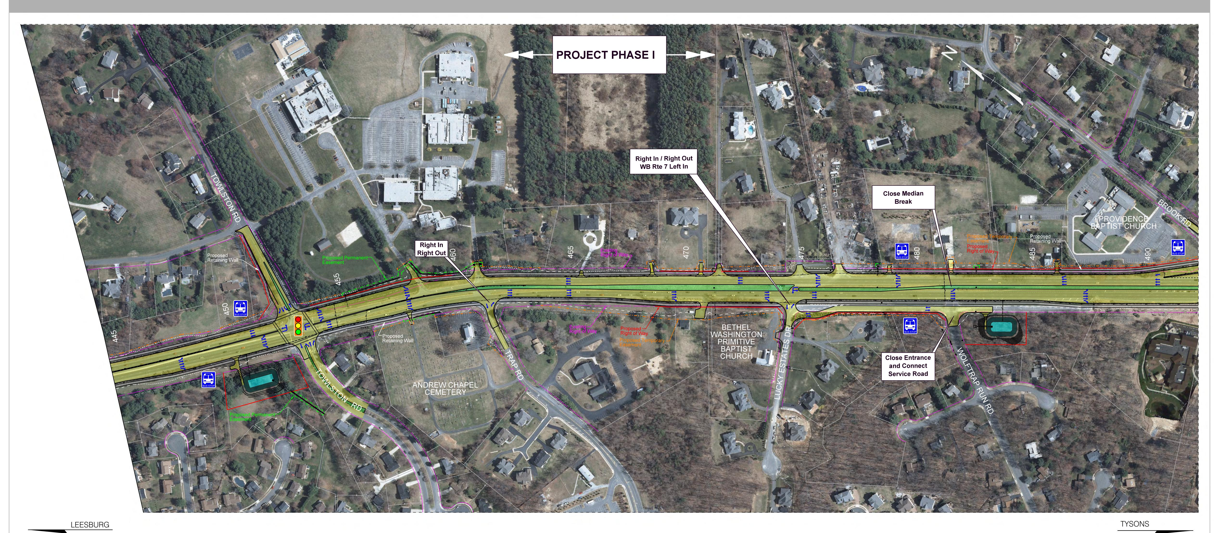
Legend Proposed Road ----- Construction Limits in Cut – – Construction Limits in Fill Proposed Bridge Proposed Shared Use Path ··-··- Proposed Temporary Easement Proposed Preliminary Stormwater Management Basin ---- Proposed Permanent Easement
